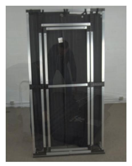
**Please note:** Hang the blankets on the inside of the frame. Start from the middle of the door and follow around until you get back to the door. No need to stretch the blankets they should hang loose.
