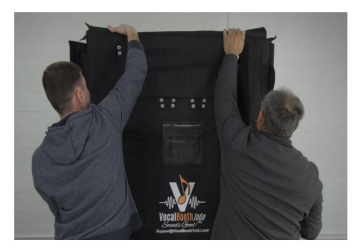
**Please note:** Start by hanging the Door panel same way as the wall panels. Then adjust the position to make sure that the door frame fit and the door can open. You would need to place the metal hook brackets of the door panel over the plastic F connectors of the door frame.
