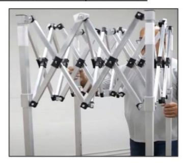
NOTE: When expanding the frame make sure to expand evenly in all directions, so the parts do not skew and get stuck. When fully expanded, make sure it is locked in place.
