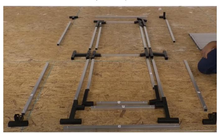
Start assembling top parts (start with the bar labeled as E on the picture)
