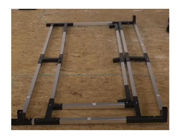
Complete the booth frame assembly. Stand the booth frame upright and add the Swinging portion of the door
