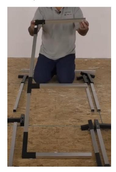
Insert the C bar into the F connector
