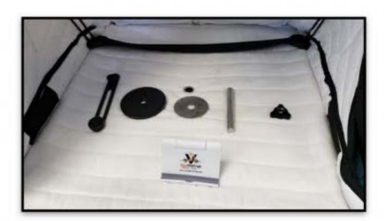
3) Prop open booth by pulling the inside black strap towards you, aligning it with the black rectangles on the sides. This puts the canopy in the proper place for full booth
